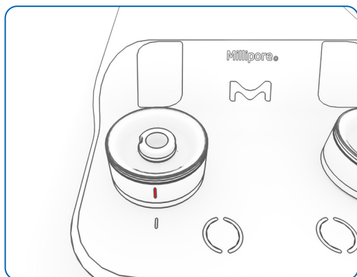
Figure 47: the sign on a locked head is aligned with the one on the pump body
