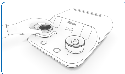
Figure 27: membrane support removal by twisting it
