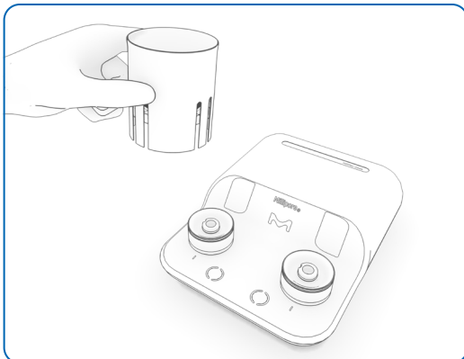
Figure 29: membrane support removal with removal tool — part 2
