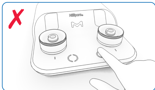
Figure 4: INCORRECT – no activation if the finger touches the outer ring
