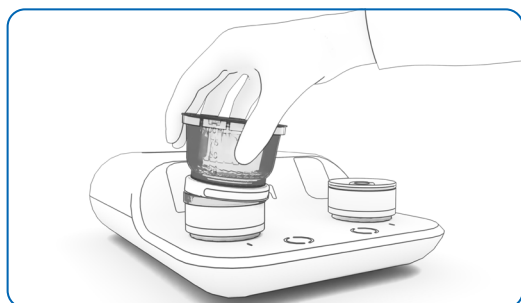
Figure 19: Filtration unit tilted for removal
