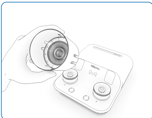
Figure 30: membrane support removal with removal tool — part 3
