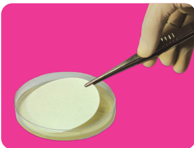
Fig 2. The membrane is placed onto the agar on which colonies have grown.
