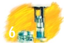
After the sample has been prepared for introduction onto the LC column, analysis can begin. Judgements based on analyte concentration require a reliable quantity of sample volume. The process of introducing the sample onto the column with precision syringes can be automated for increased throughput.<sup>39, 40</sup>
