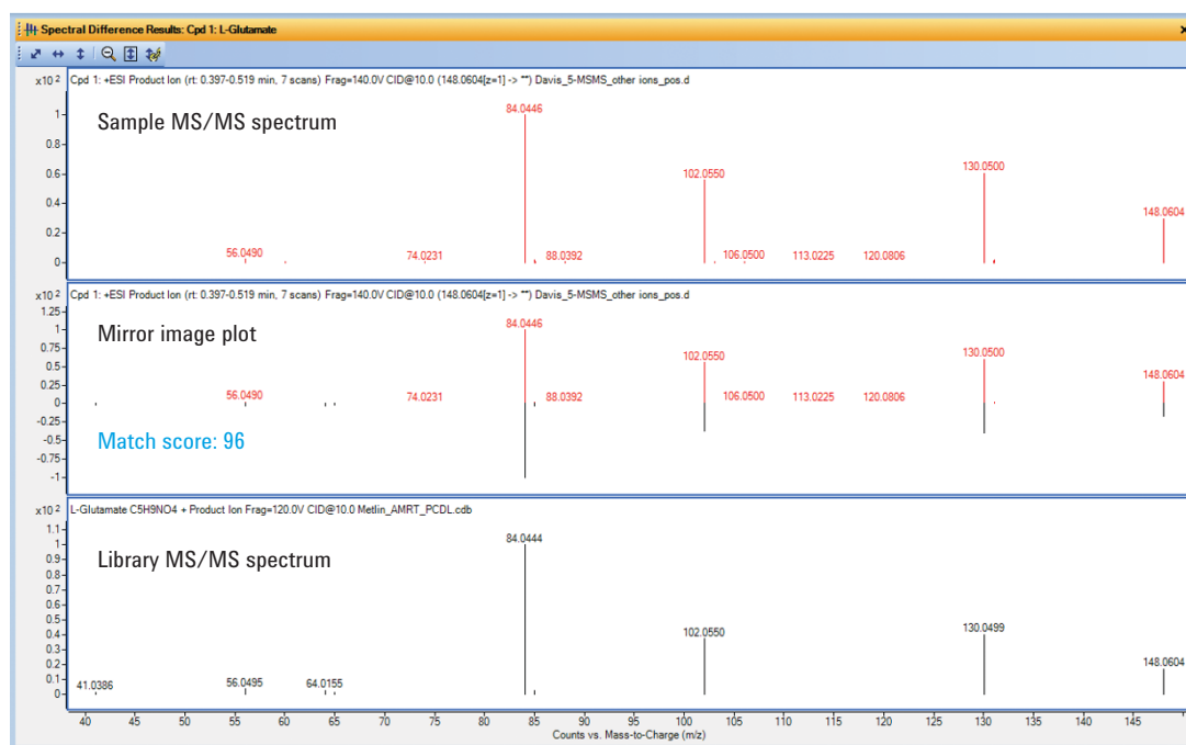
Figure 11A. Compound identification using LC/Q-TOF MS/MS spectra matching with a reverse score of 96 for L-glutamate in positive ion ESI mode. The reverse score reflects ion matches for those peaks from the library standards that are reflected in the spectrum acquired from the sample. The collision energy (CE) of 10 eV was used to acquire the sample MS/MS spectrum.
